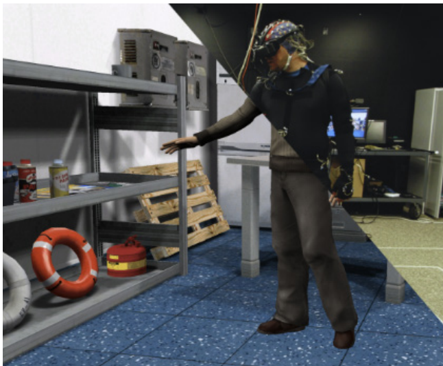
A subject interacting with a virtual reality environment while wearing EEG sensors in the MoBi lab (mobile brain and body imaging)
